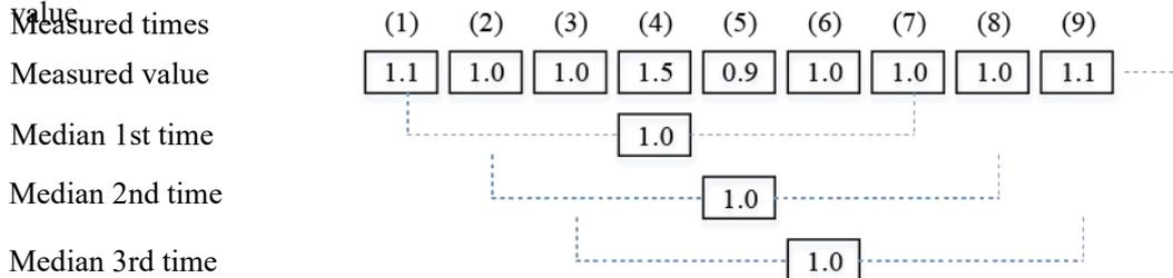
For example, when the median is executed for the first time, the order from (1) to (7) becomes the following, with the central value of "1.0" being the measured value.
