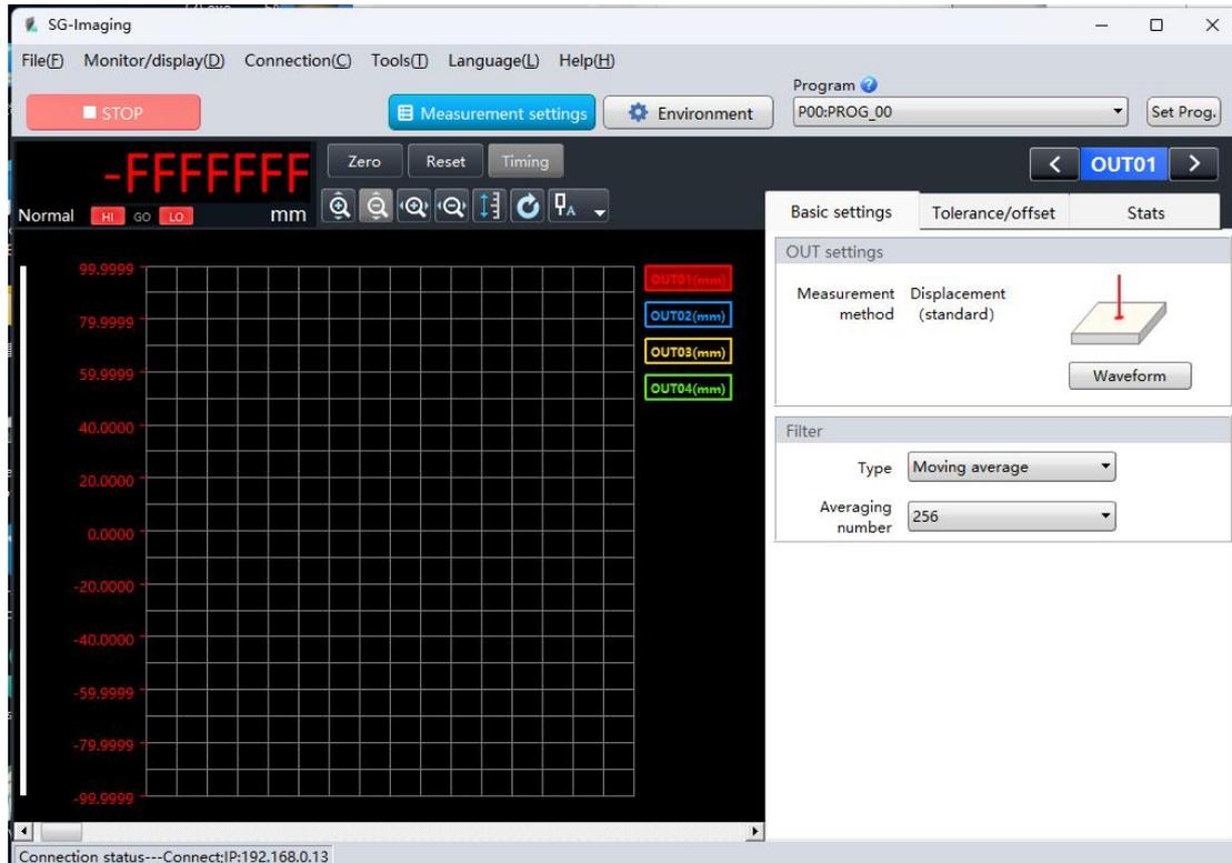
If the connection to the controller fails, please click [PC Communication Settings] to confirm if the IP address of the controller is correct.
