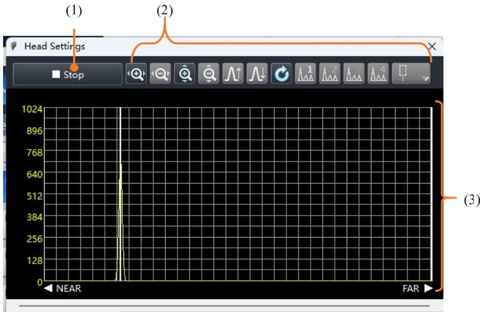
When the measurement method is for transparent object 2, it can display the photosensitive peak waveform after processing four ABLE values.
