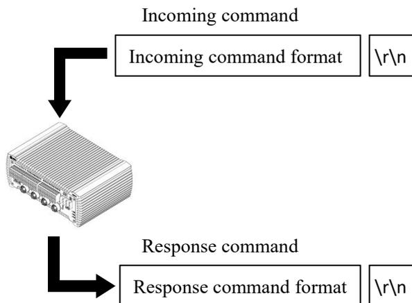
**Note:** When creating a control program, the program built should allow you to send the next command after confirming that you have received a response command from the sensor.
