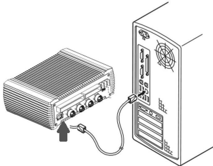
1. Insert a commercial Ethernet cable (CAT-5 crossover cable) into the Ethernet interface on the controller.
