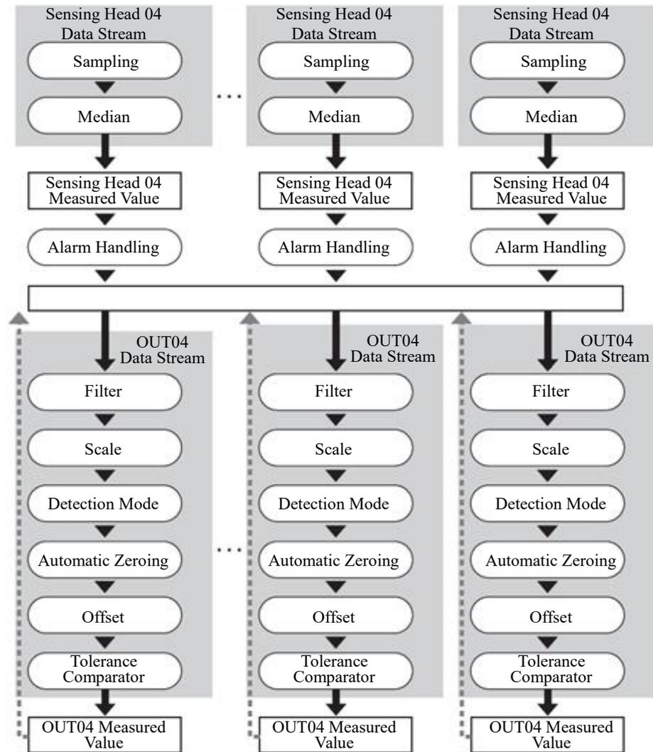
The measurement values from OUT01 to OUT04 can be used up to three times in the calculation.
